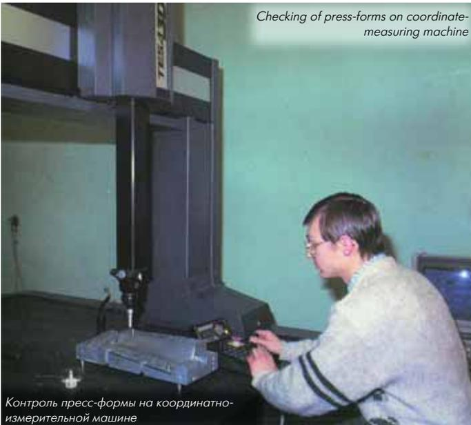
Checking of press-forms on coordinate-measuring machine
